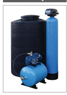
This unit removes iron and manganese to a combined level of 10 milligrams per litre The pH of your water must be 7.5 or over.
